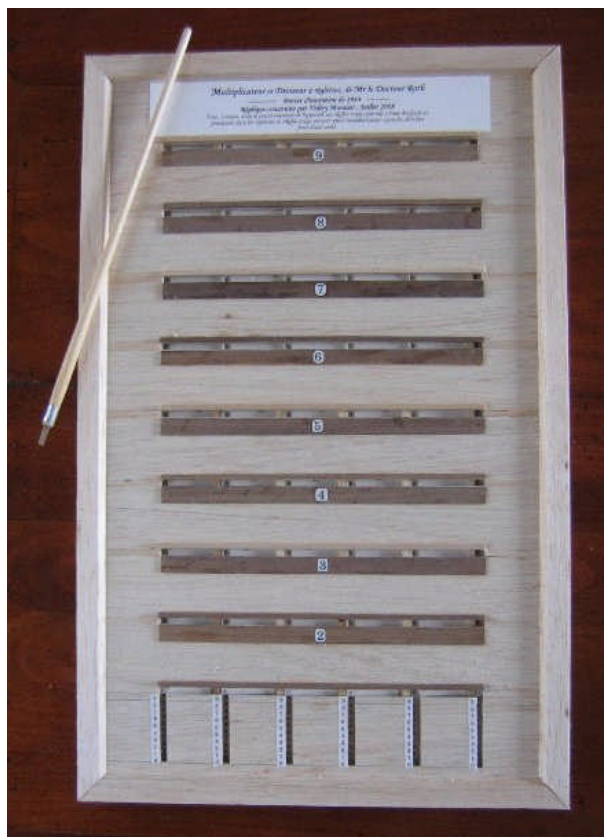
Roth's Multiplicateur et diviseur à réglettes Replica and photo by Valéry Monnier, with his kind permission
